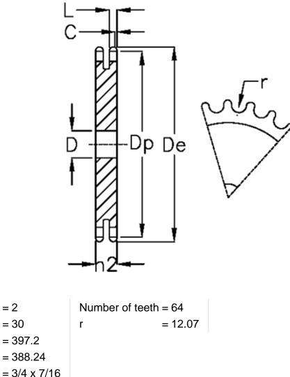
C = 2 D = 30 De = 397.2Dp = 388.24For chain size =  $3/4 \times 7/16$ For chain type = 12 B-2h2 = 30.3L = 10.8
